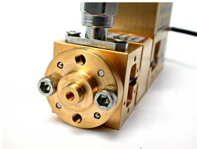
Figure 12. Detail picture of the HM-wr1.2-FB detector head equipped with a scalar (corrugated) horn.
