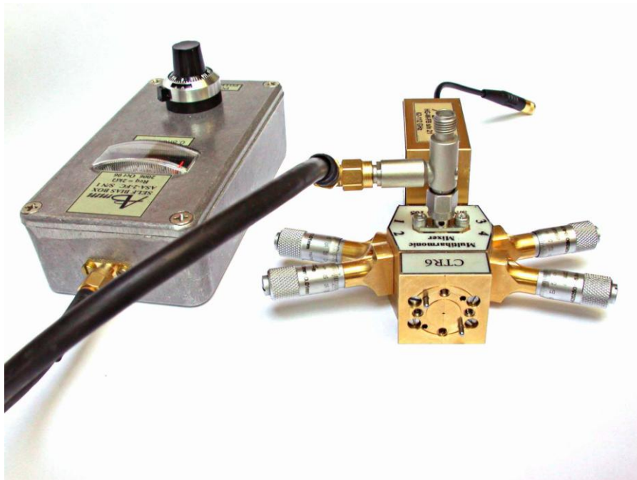
Figure 9. The ASA-2-FC extension for signal detection at 250-1000 GHz . Upon mechanical tuning to the central frequency desired the typical electronically-tuned sweep spans over 10-20 GHz.
