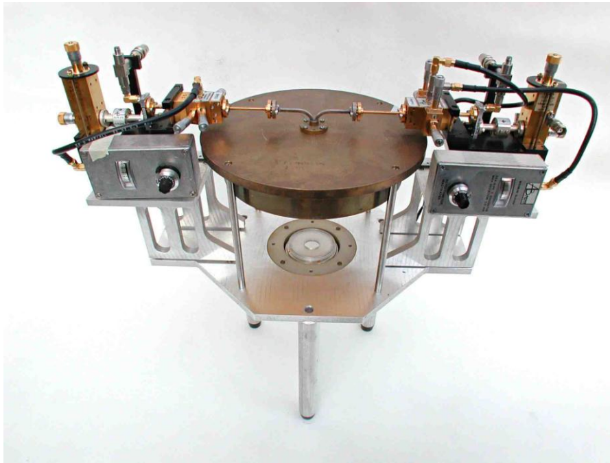
Figure 27. The Fabry-Perot submillimeter resonator shown together with the signal source, the detector and coupling waveguides. The sample is usually placed at the flat, bottom, mirror. Please note that the position of bottom mirror is adjustable.
